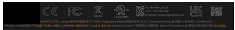
Hybrid traditional/e-label, able to better fit on the device with a QR code that is scannable, linking to a website with clear and legible regulatory information.
